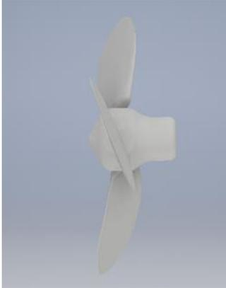
Gambar 1. model *Propeller Pitch 20°* tampak samping
