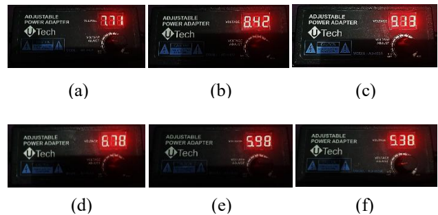
Gambar 6. Variasi Tegangan Input Menggunakan Adjustable Power Supply (a) Overvoltage 1, (b) Overvoltage 2, (c) Overvoltage 3, (d) Undervoltage 1, (e) Undervoltage 2, (f) Undervoltage 3
