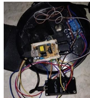
Gambar 1. Proses Perakitan Sistem Monitoring Lifetime Lampu Infrared
