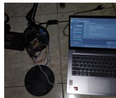
Gambar 2. Proses Upload Program ke Mikrokontroler ESP8266
