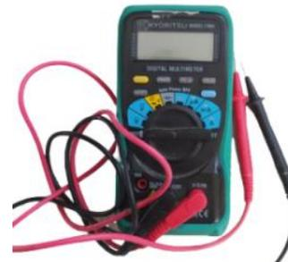
Gambar 2. Multimeter Digital
