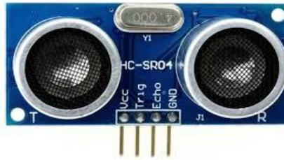
Gambar 2.3 Sensor Ultrasonik [5].
