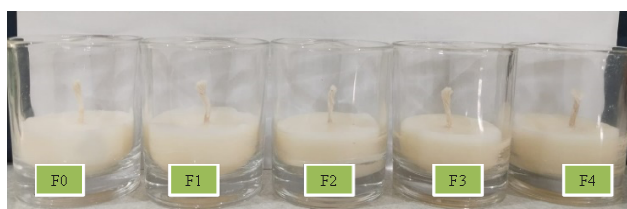
Figure 1. Aromatherapy candles made from keruing oleoresin (F0: Oleoresin 0%; F1: Oleoresin 2,5%; F2: Oleoresin 5%; F3: Oleoresin 7.5%; F4: Oleoresin 10%).
