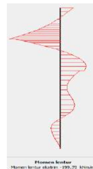
Gambar 13 Momen Diaphragm Wall Sumber : Output Plaxis
